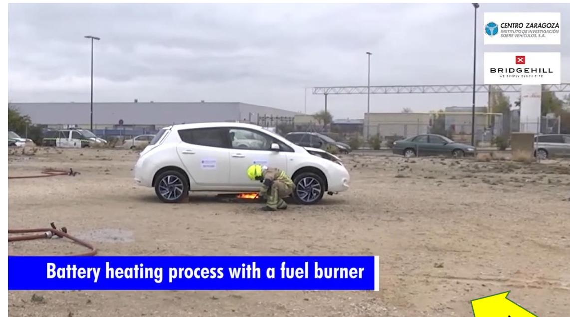
Battery heating process with a fuel burner
